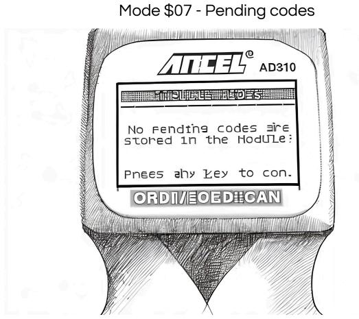
The pending codes are a bit different. It's only triggered if the fault is detected a certain number of times in a certain number of drive cycles. The number of recurrences and drive cycles can vary depending on the fault.
