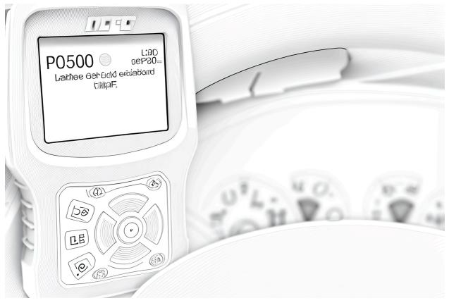
The most basic function of OBD2 scanners is reading fault codes. There are thousands of different OBD2 codes, and each of them is triggered if some test fails. These codes are not just random numbers and you can get a lot of insights from general rules that apply to all codes. First of all, there are different types of OBD2 Codes:
