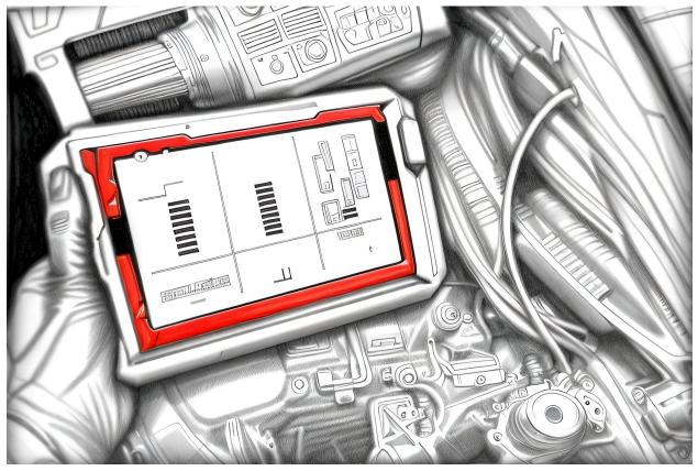
Bi-directional testing is another cool feature of advanced scan tools. It's like having a conversation with your car. Instead of just reading info from the car, you can also send commands to it. This helps you test different parts without physically touching them. For example, you can tell the fuel pump to turn on and off or make the cooling fans spin. This is super helpful for checking if things are working right.
