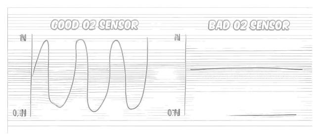
Every gasoline car has at least 2 oxygen sensors. Sensor 1 is before the catalytic converter, and sensor 2 is after the cat.
